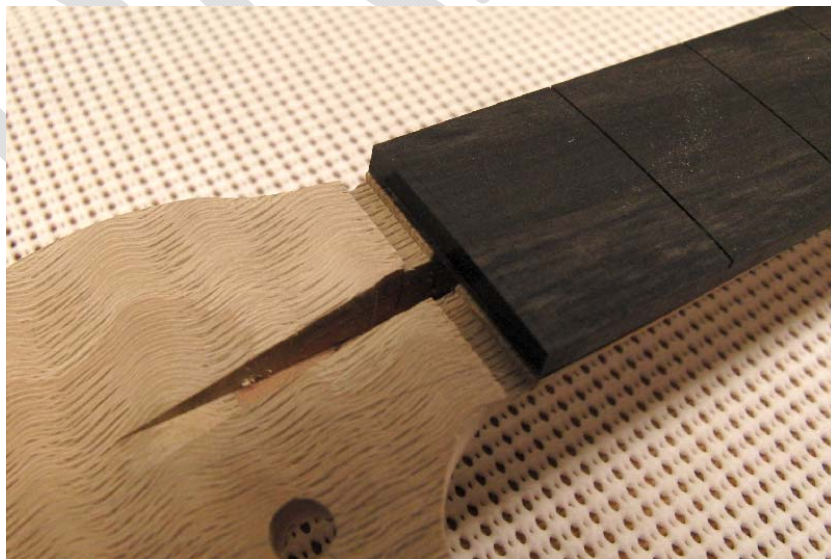
Figure 19 – Fretboard Correctly Aligned on Neck
