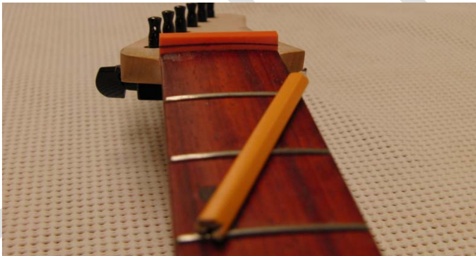
Figure 47 – String Nut with the Radius Marked Correctly
