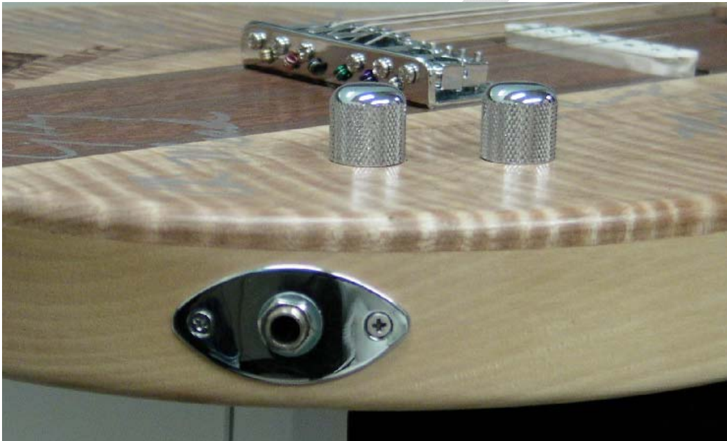
Figure 40 – Jack Plate Secured to the Body
