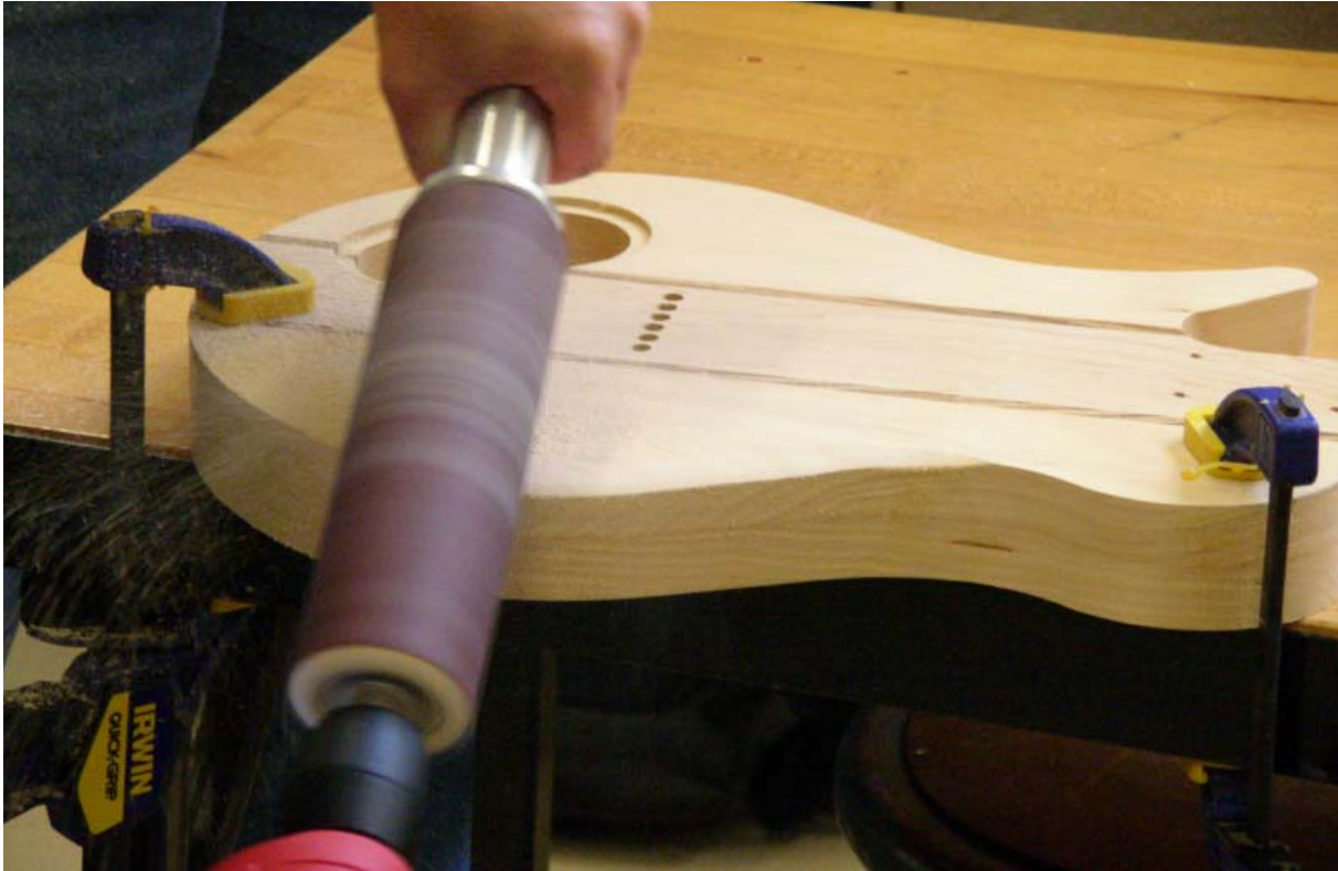
Figure 5 – Contouring a Body Using a Pneumatic Sanding Drum
