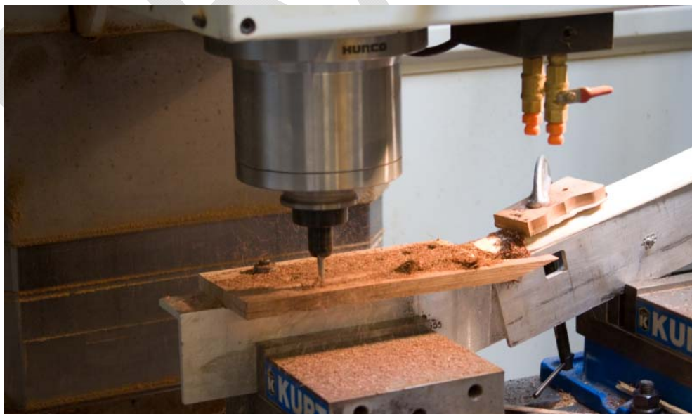
Figure 11 – Headstock Being Milled
