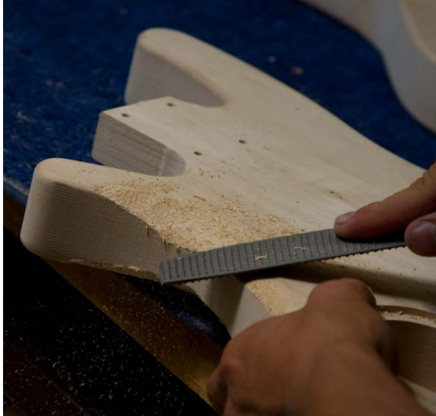
Figure 6 – Shaping a Body with a Rasp
