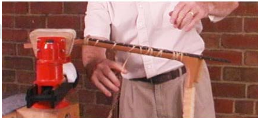
Figure 21 – Heavy Rubber Bands Being used to Clamp a Fretboard to a Neck (picture courtesy of Stewart MacDonald, www.stewmac.com )
