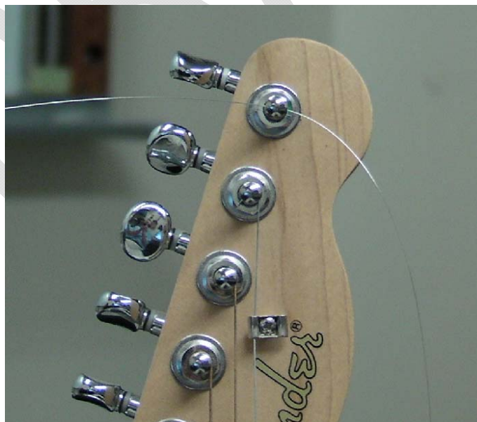
Figure 55 – Inserting Plain String through Hole in Tuner Post
