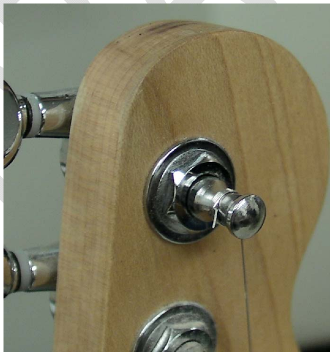
Figure 59 – Trimmed End of String (Sharp!)
