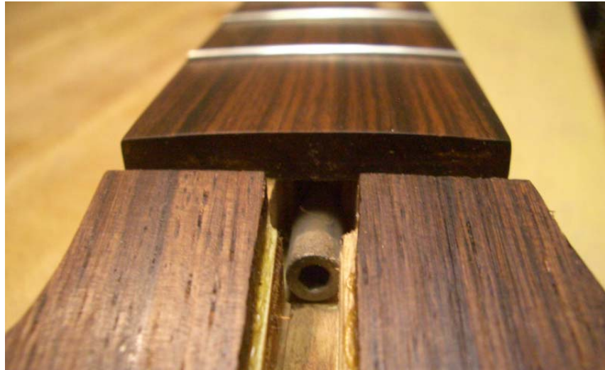
Figure 18 – Correct Truss Rod Orientation with Nut at Bottom of the Slot
