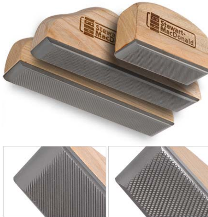
Figure 32 – Files Used for Leveling Frets and Fretboards (image courtesy Stewart MacDonal, www.stewmac.com )
