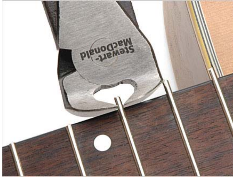
Figure 31 – Trimming the Fret Ends Flush (image courtesy of Stewart MacDonald, www.stewmac.com )
