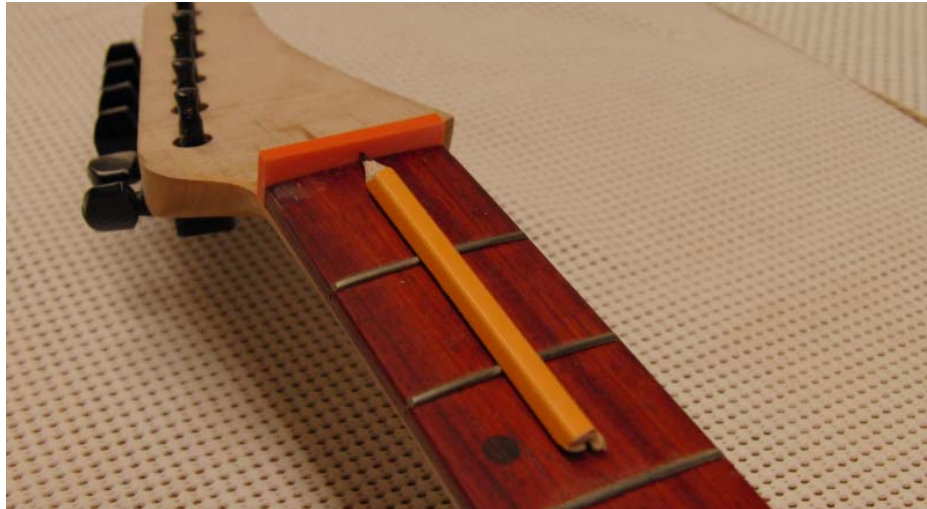
Figure 46 – Marking the Neck Radius on the Nut
