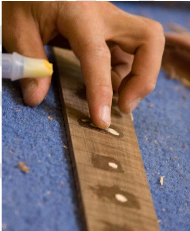
Figure 16 – Gluing Wood Dots into the Fretboard
