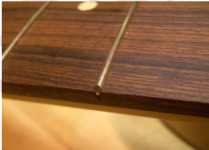
Figure 35 – A Correctly Dressed Fret End
