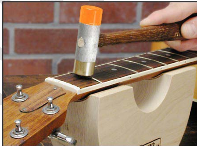
Figure 28 – Seating the Center of a Fret with a Fretting Hammer (image courtesy of Stewart MacDonald, www.stewmac.com )
