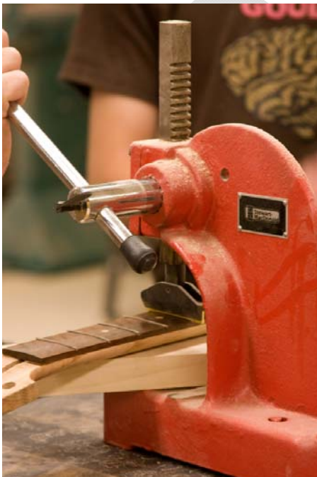
Figure 27 – Arbor Press for Installing Frets (image courtesy Stewart MacDonald, www.stewmac.com )
