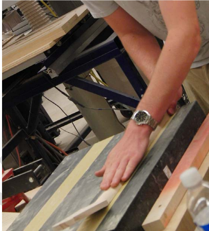
Figure 17 – Flattening Neck Before Gluing on Fretboard
