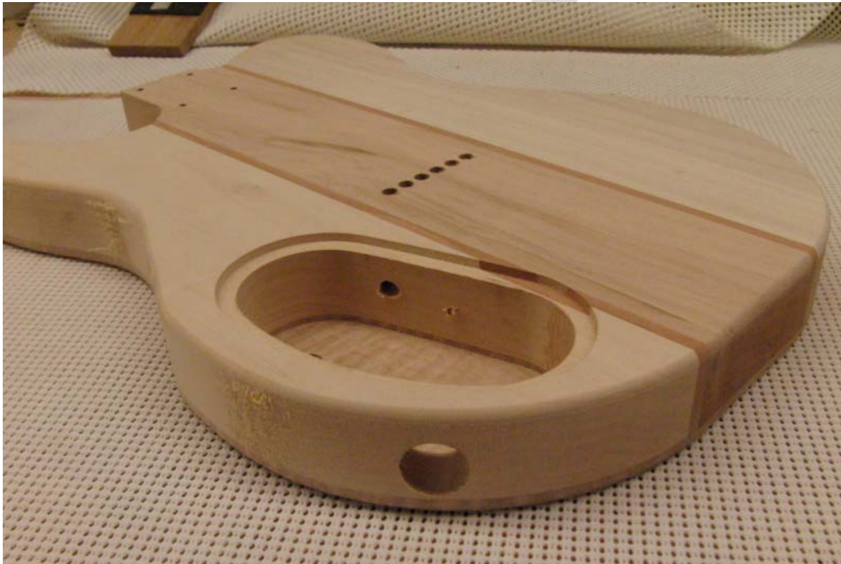
Figure 2 – Guitar Body with Body Radius and Holes Drilled
