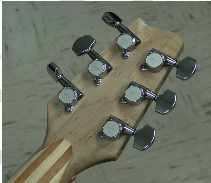
Figure 42 – The Back of a Headstock Showing the Small Set Screws
