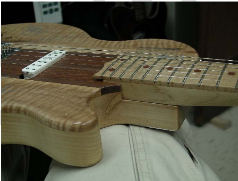
Figure 44 – Neck Properly Seated In Pocket
