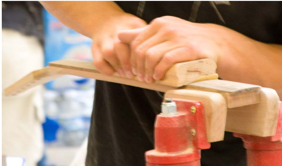
Figure 23 – A Short Radius Being Used to Level a Fretboard
