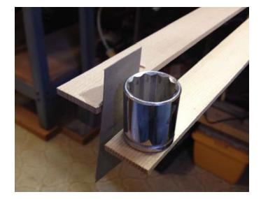
Aside: Wood displays a property known as *creep*, which means that a sample will continues to deflect slowly after a load is applied. The beams used in this experiment may creep when loaded, so you may notice that your test beam continues to move just a little. Rather than try to wait until it stops creeping, record the deflection right after applying the load.
